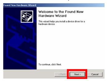
2. The USB 2.0 driver should come from your computer's system drivers; it is not a part of the docking station's driver. The user must have the computer's system drivers ready and specify their path to the installation wizard. Select Specify a location and click **Next** to proceed.
